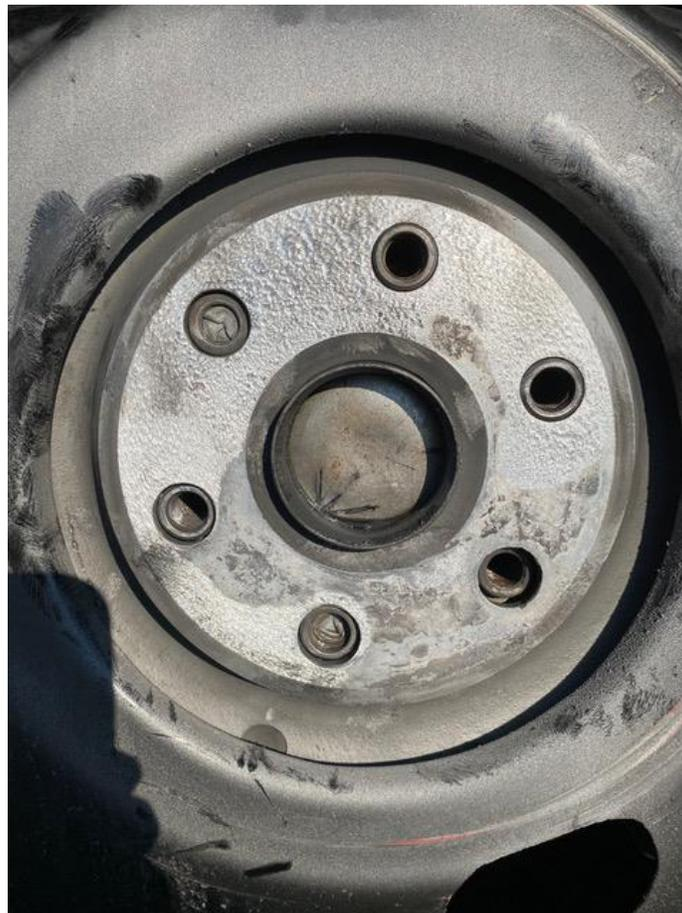
**Front view of crankshaft propeller hub.**
