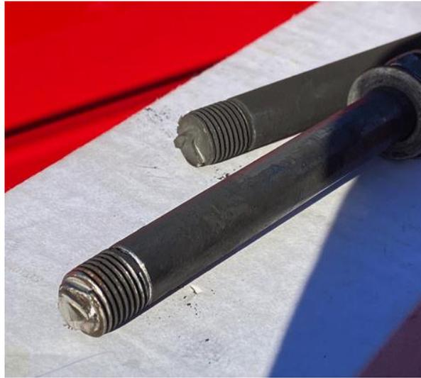
**Fractured propeller bolts**
