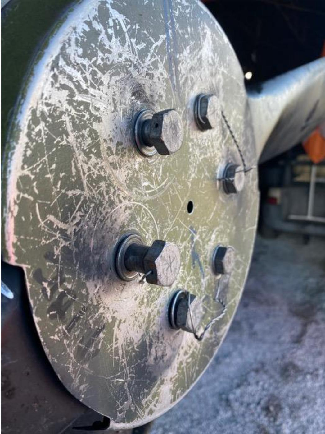
**Spinner plate on front of the propeller hub**
