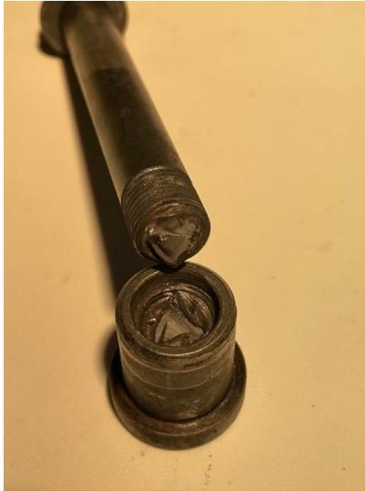
**Fractured bolt and companion bushing/nut.**
