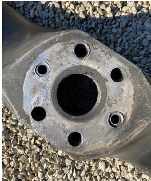
**Damaged propeller hub**
